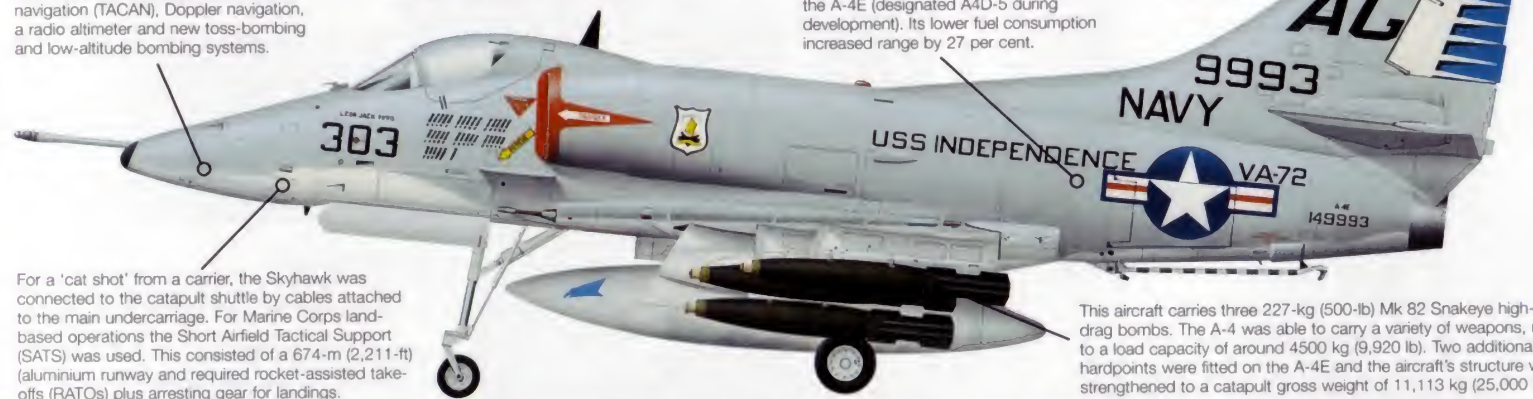
Essentially a 'cropped delta', the A-4's wing span was just 8.38 m (27 ft 6 in). This meant that a folding wing was not required for storage aboard an aircraft-carrier.
